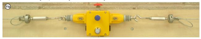
12. Tighten the lock nut tightly to the hexagon adjuster.
