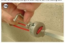
11b. For optimum performance the switch tension should be set at mid position (as indicated by the markers in the viewing window).
